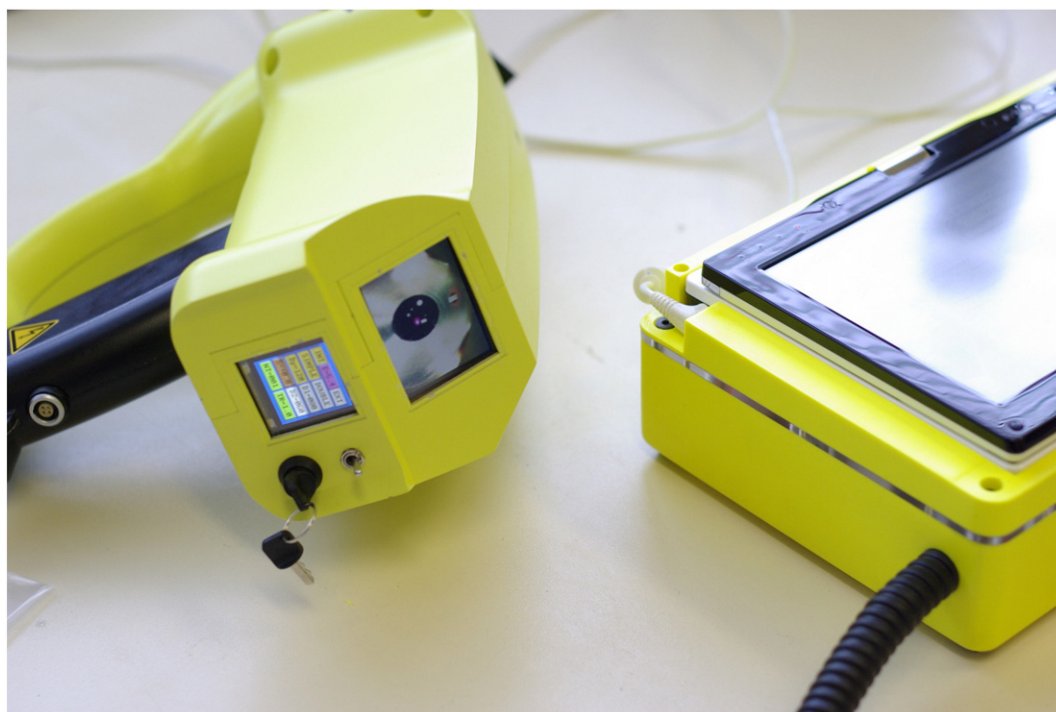
Fig. 1. Portable LIBS system and its two main parts, connected together with the umbilical.
