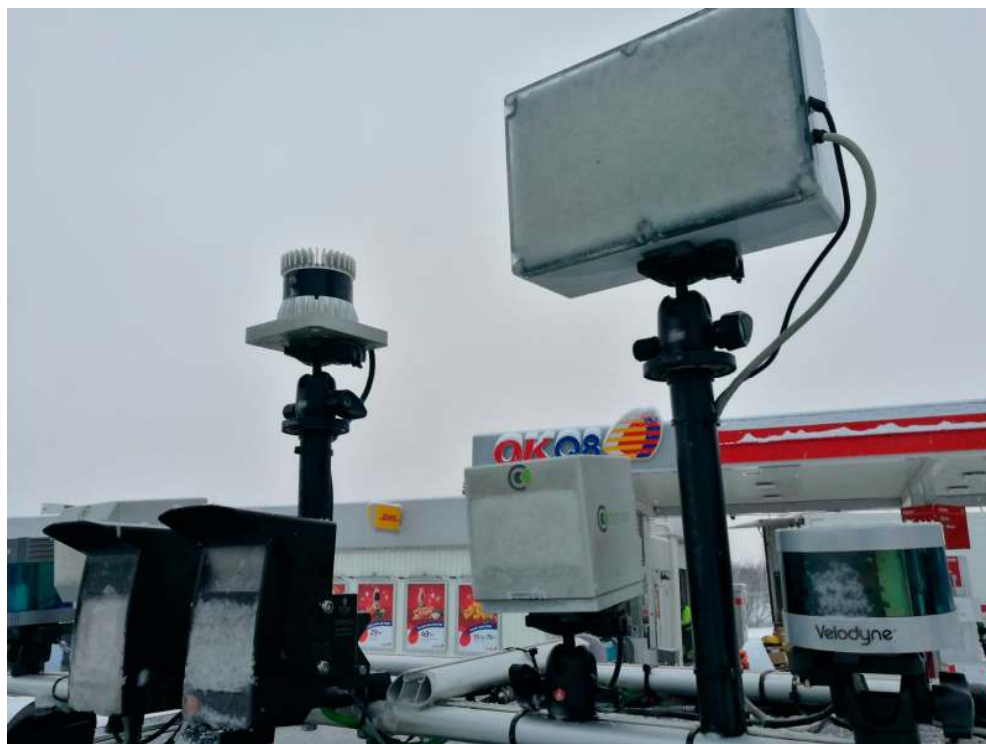
Figure 3. Frozen sensors when the temperature is less than -15\text{ }^{\circ}\text{C} .
