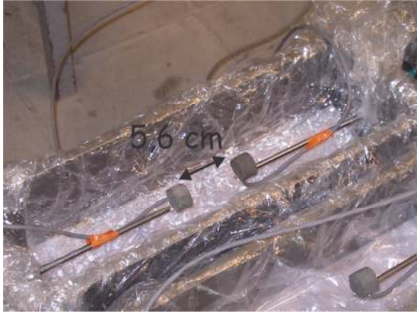
40 Figure 12: Prismatic mould with SMAGs before casting the concrete.
