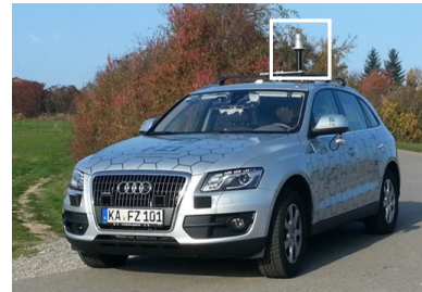
Fig. 5: FZI’s Cognitive Car: On-board reference sensors, like a high resolution laser scanner, facilitate referencing less accurate sensors.
