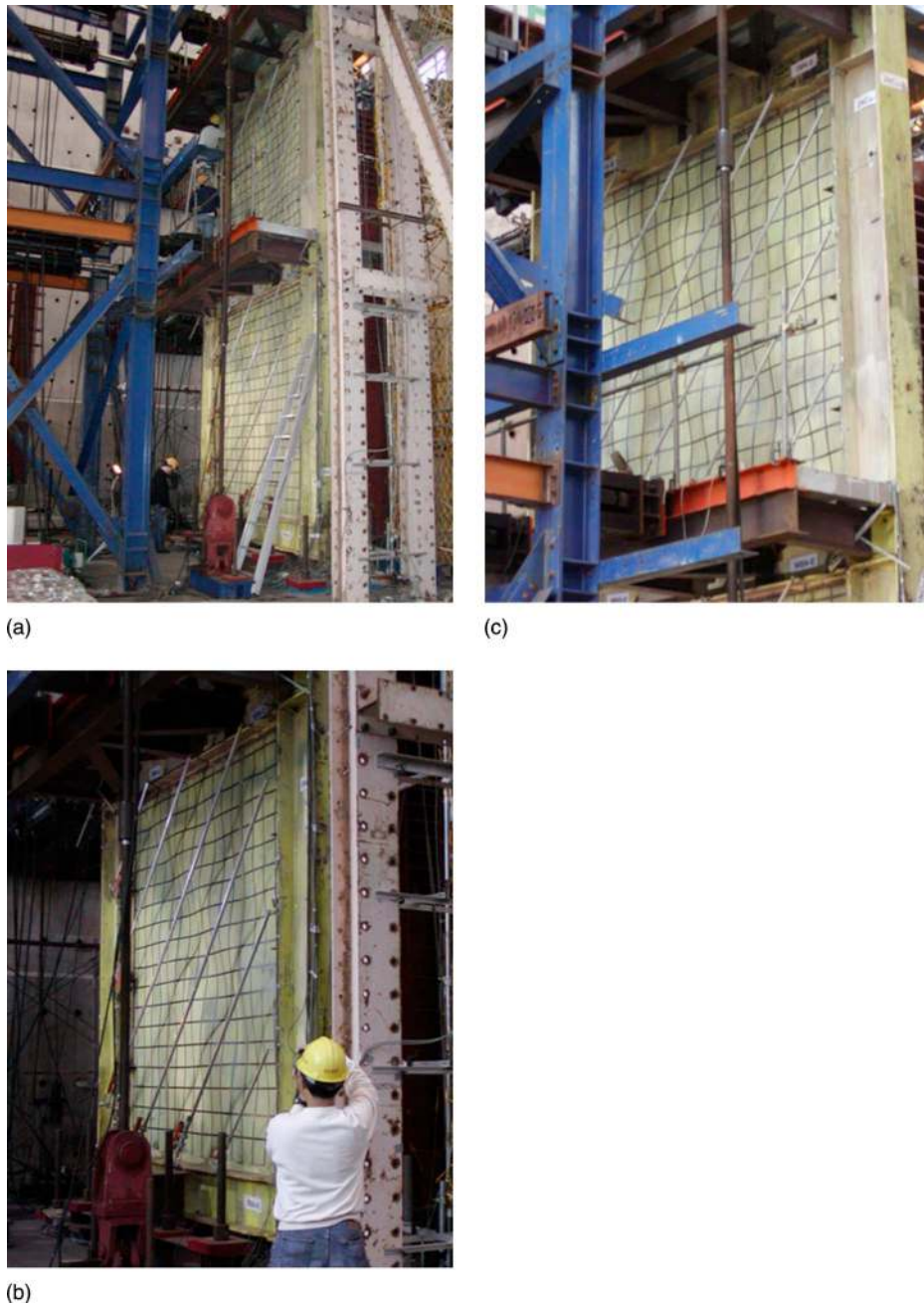
Fig. 6. Deformed specimen and buckled panels in Phase II pseudodynamic test: (a) specimen; (b) 1F panel; and (c) 2F panel
