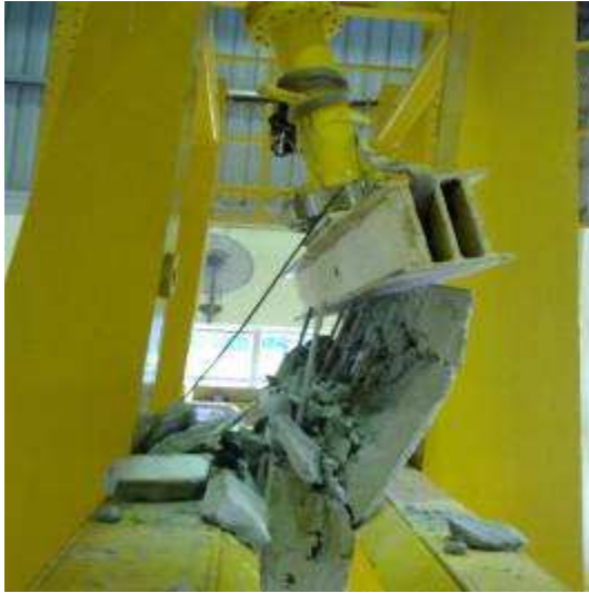
Fig. 22: Crushing at the Top Part of Panel 2
