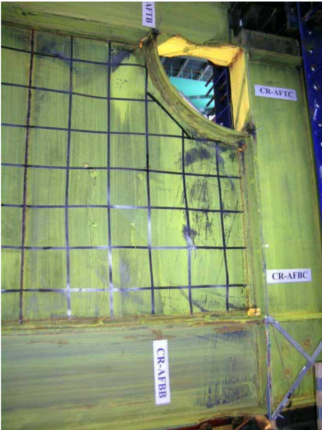
Figure 9: Infill panel and RBS yielding (Specimen CR: Cycle 19, \gamma = 1.5\% \approx 5\delta_y )
