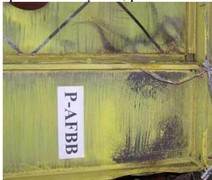
Figure 7: Yielding of bottom beam RBS (Specimen P: Cycle 23, \gamma = 2.5\% \approx 8.333\delta_y )
