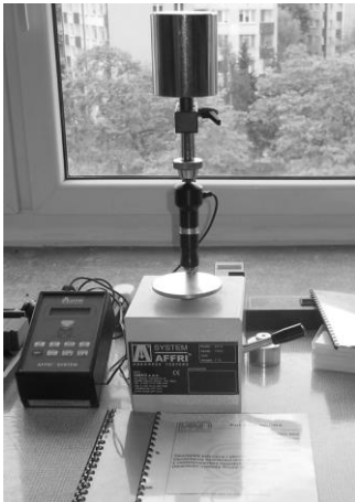
Fig. 5. Scheme of hardness measurement stand (with the use of Shore's method A)
