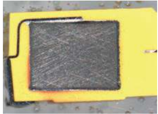
FIGURE 9: A cross-section of a failed capacitor.
