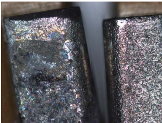
FIGURE 3: Capacitor after 96 h in salt spray (left) and a nontested capacitor (right).
