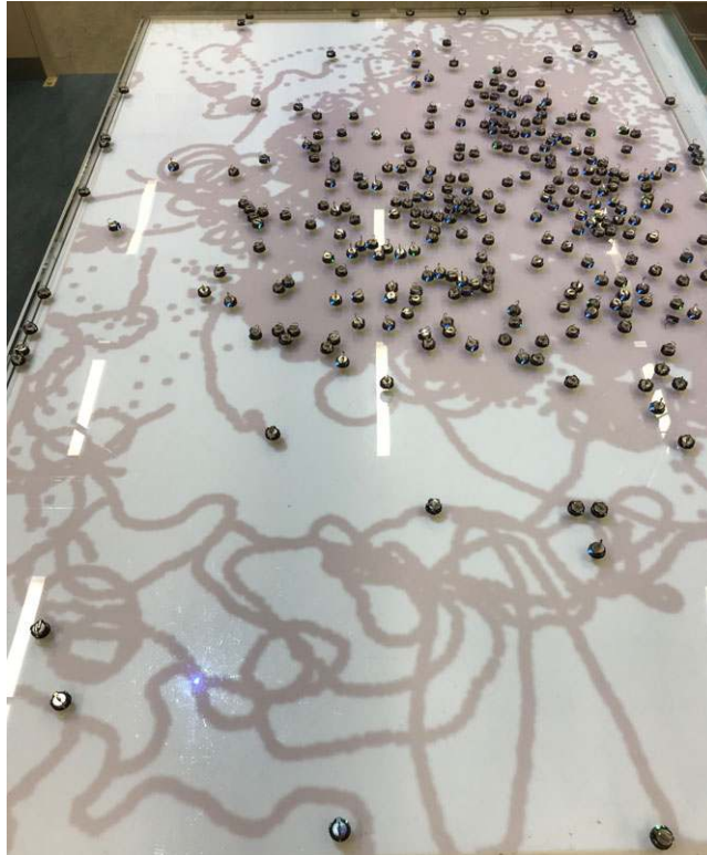
Figure 1. Arena at T = 15 min, N = 324 Kilobots in the trail avoidance (stigmergy) condition. A large patch of repellent pheromone has formed.
