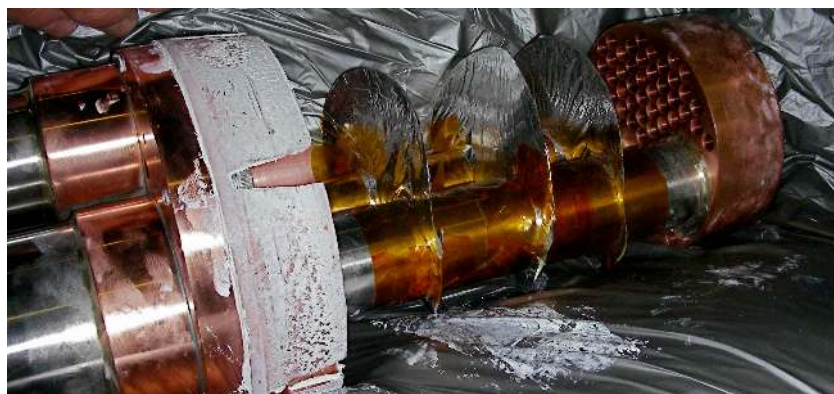
Figure 4. First Stage Pressed Tapered Fit (left), Second Stage Condenser (right), and Baffles between the Stages
