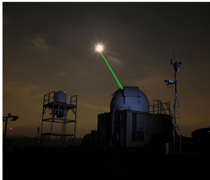
Figure 10: NASA's NGSLR system is being used to laser range to the Lunar Reconnaissance Orbiter (LRO) orbiting the moon [33]. (Image credits: Tom Zagwodzki / GSFC.)
