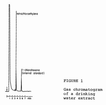
During a period of 12 days, the levels of tetrachloroethylene were determined on a daily basis. In addition, the analyses of deionized, doubly-distilled, and UV irradiated (24 h, 254 nm) water showed that these three water purifications did not completely remove tetrachloroethylene. Tap water from another location at Dubendorf (location A, Table 1), however, contained much smaller amounts of tetrachloroethylene than the tap water at EAWAG. Table 1 summarizes the data.
