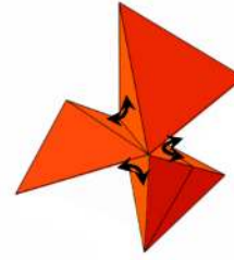
Figure 2: Edge-adjacency of cut-border triangles around non manifold edge.
