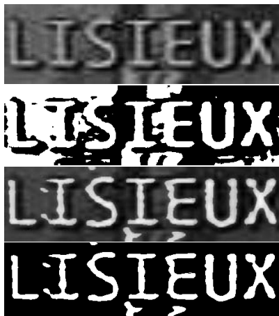
Fig. 5. (a) original image. (b) binary image. (c) enhanced image. (d) binary enhanced image
