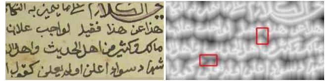
Figure 5: A document image and its distance transform, where two fork examples are marked with red rectangles.
