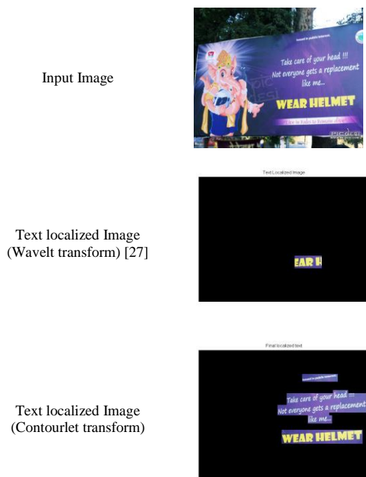
Fig.6. Performance Comparison of the Proposed Method Based on Contourlet Transform and the Method in [27]
