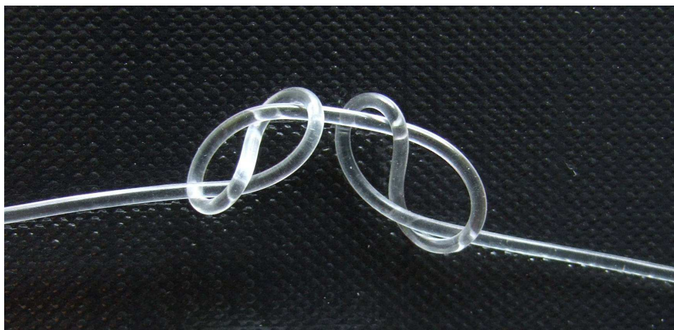
Figure 2. Extruded silicone fiber of 0.51 mm core diameter.
