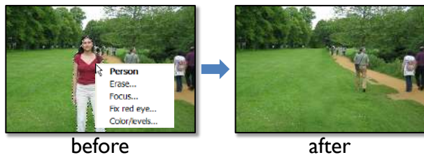
Figure 24: Semantic-aware interactive image editing. Left: the semantic segmentation given by TextonBoost is used to drive a semantic-aware user interface. Here the user has selected the person, and a context sensitive menu presents editing options specific for the ‘person’ class. Right: after the user clicks ‘Erase...’, an automatic system [11] removes the person from the image by filling in over the top of her.
