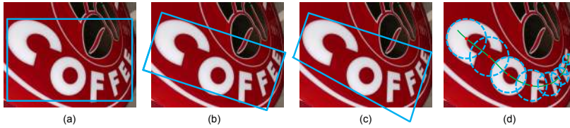
Fig. 1. Comparison of different representations for text instances. (a) Axis-aligned rectangle. (b) Rotated rectangle. (c) Quadrangle. (d) TextSnake. Obviously, the proposed TextSnake representation is able to effectively and precisely describe the geometric properties, such as location, scale, and bending of curved text with perspective distortion, while the other representations (axis-aligned rectangle, rotated rectangle or quadrangle) struggle with giving accurate predictions in such cases.
