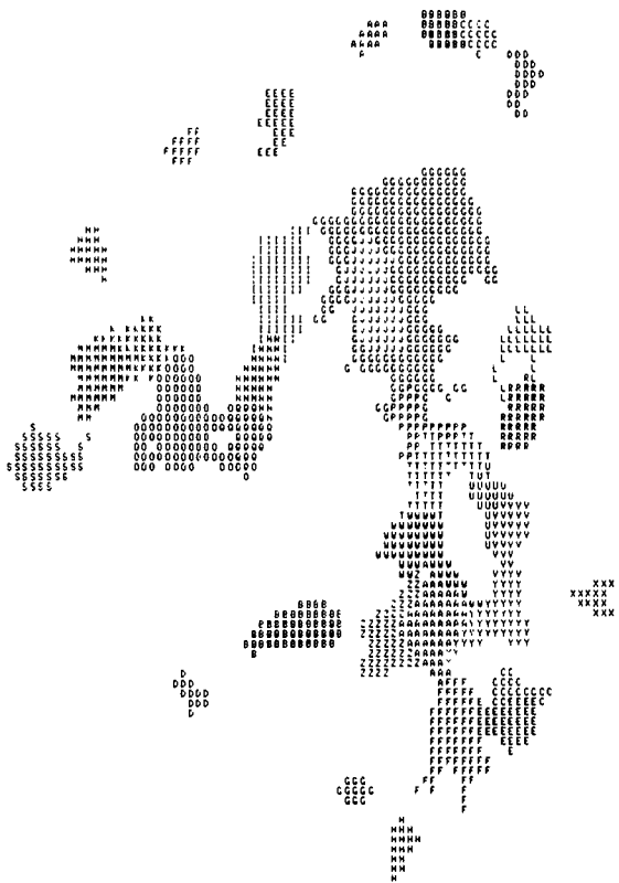
FIG. 2. Line printer representation of the segmented regions with relative high chromatin contrast found by the region grow algorithm in the digitized image of the nucleus shown in Figure 1. The area of the individual segments is marked by a character indicating the sequence in which the segments are found. The vertical elongation of the picture is caused by the line printer format.
