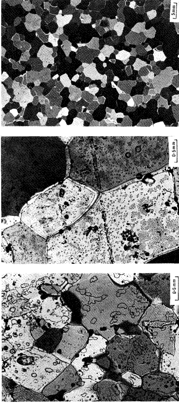
a b c FIGURE 4 Microstructures associated with ice sample 10-4. (a) micrograph at completion of deformation. (b) micrograph of sample annealed at -1^{\circ}\text{C} for 2 days. (c) annealed at -1^{\circ}\text{C} for 32 days.
