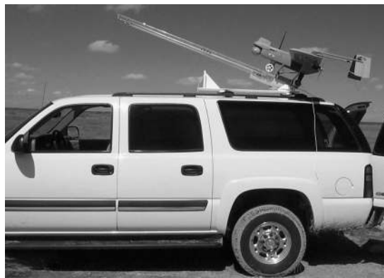
Fig. 1. BAT 3 UAV on catapult launcher ready for takeoff.
