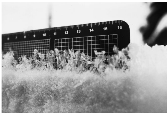
Fig. 5. Surface-hoar crystals on surface near Mount Fidelity, British Columbia. Photograph taken on 28 December 1995 a few hours before burial. Some results of monitoring this layer after burial are shown in Figure 6.
