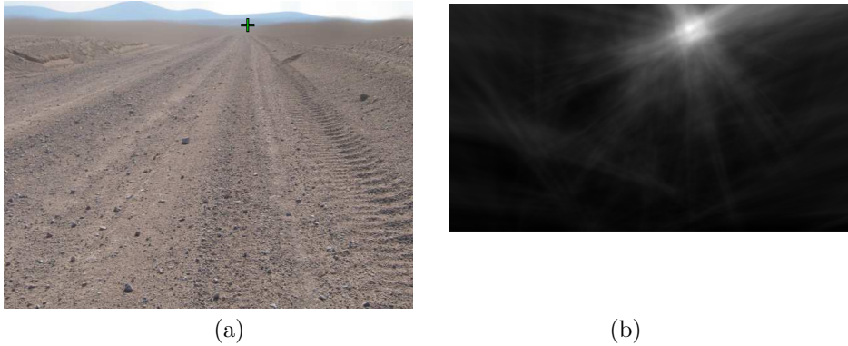
Figure 1: (a) Desert road from DARPA Grand Challenge example set (with vanishing point computed as in Section 2.1); (b) Votes for vanishing point candidates (top 3/4 of image)
