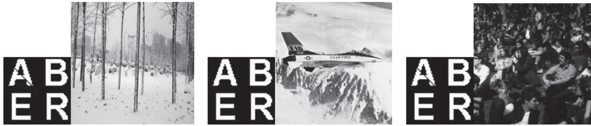
FIGURE 6: Extracted watermarks from attacked images ( Snow , Plane , and Crowd ) after a scaling attack (scale = 1/2).
