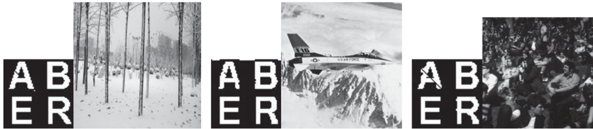
FIGURE 7: Extracted watermarks from attacked images ( Snow , Plane , and Crowd ) after a JPEG attack (JPEG = 40).
