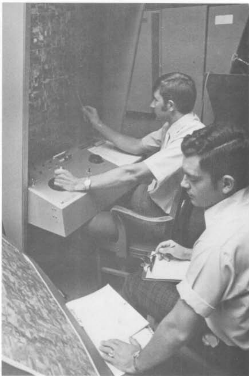
Figure 6. Most of the 210 segments in the 1971 Corn Blight Watch Experiment were analyzed using a Variscan rear-projection system for photointerpretation. Results were reported and rushed every two weeks to Washington.
