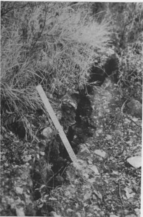
Fig. 5. Details of the fault break south of Eleochori road (site 5 on Figure 2b). Figures 5a, 5b and 5c are at site 4; Figure 5d is at site 2 (see Figure 2b). (a) Continuous, 3-cm-wide fissure makes 10- to 12-cm-high step in soil, less than 1 m away from the N45^{\circ}E striking and 60^{\circ}W dipping fault plane in bedrock (see Figure 6). (b) As step in soil merges with bedrock/soil fault plane, the net resolved dip component of slip is 10 cm. (c) A 13-cm-high step-and-fissure 3 m away from the bedrock fault. Because of the collapse of the hanging wall, the apparent slip may be reverse. (d) Slickensides and grooves rake 82^{\circ}N on a N15^{\circ}E striking and 70^{\circ}W dipping plane. Only 6- to 7-cm-wide bare stripe at the base of the plane was exhumed by the downdrop of grass-covered sediments during the earthquake. Note that the smallest break is observed just at the foot of Mount Kalathio where the long-term displacement reaches a maximum.
