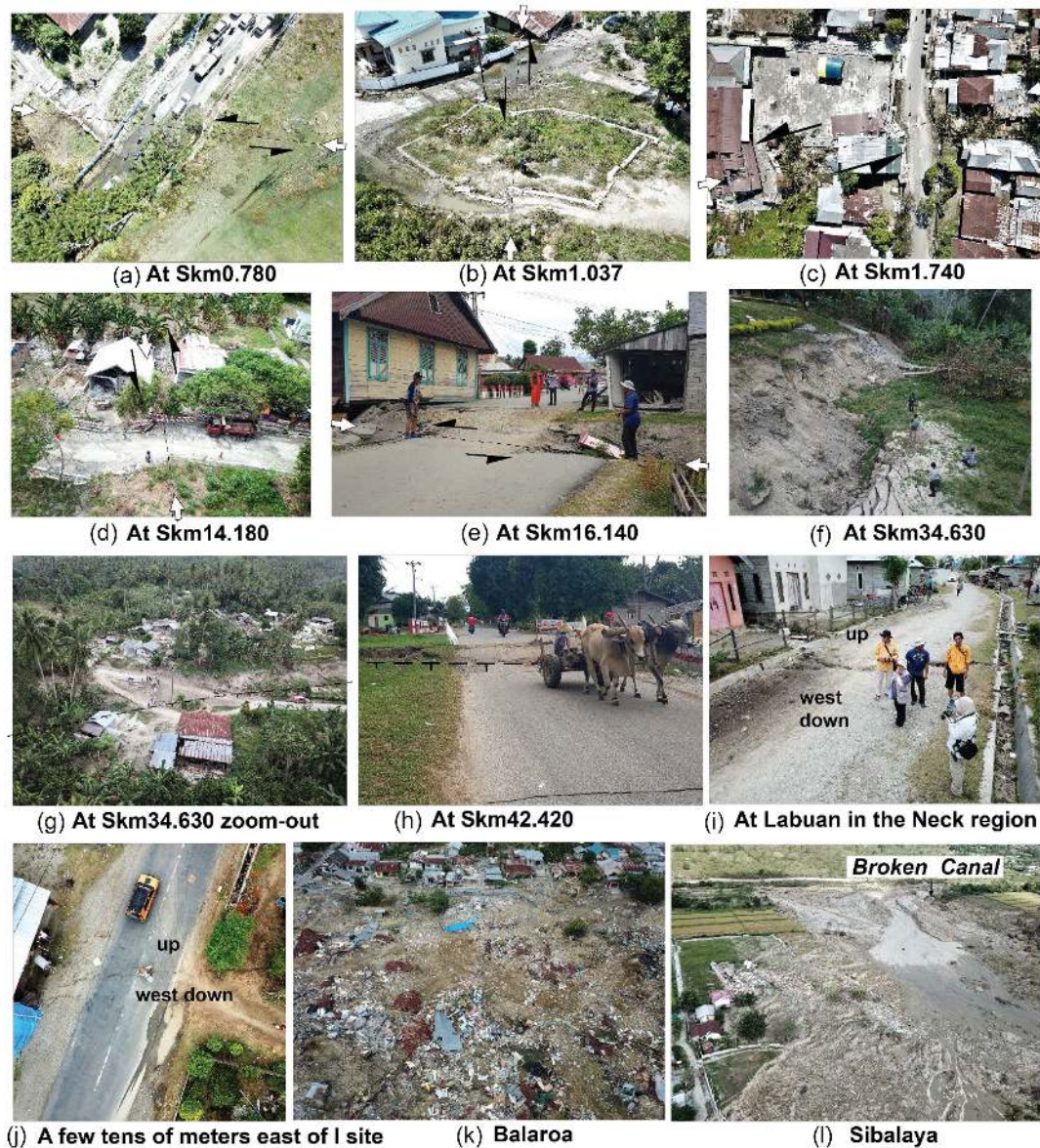
Figure 8. Field photos showing examples of fault ruptures and offsets of the 2018 event. (a) Km1 + 740, (b) Km0 + 780, (c) Km1 + 037, (d) Km14 + 180, (e) Km16 + 140, (f) Km34 + 630, (g) Km34 + 630, (h) Km42 + 420, (i) and (j) on land rupture in the eastern side of Km25 seabed—northern side of Palu City, (k) Liquefaction, and land movements in Balaroa and (l) liquefaction and land movements in Sibalaya. The location of the photos are marked in Fig. 6 and Fig. S2e in the Supporting Information.
