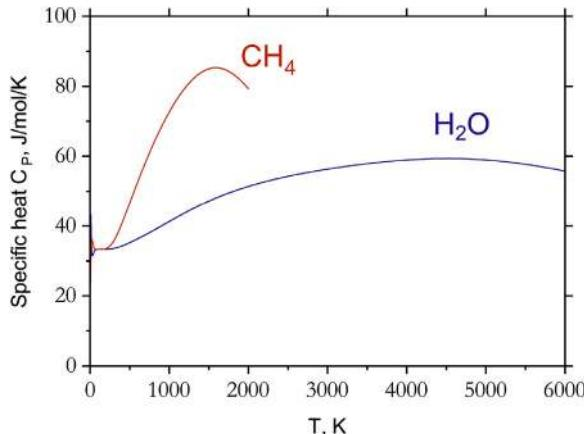
**Fig. 3.** Specific heat at constant pressure of H<sub>2</sub>O as computed by Furtenbacher et al. [259] and CH<sub>4</sub> generated the YT10to10 ro-vibrational energies [97].
