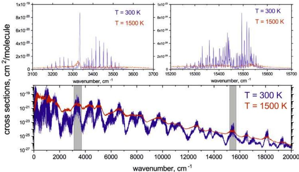
**Fig. 2.** Absorption cross sections generated using the ExoMol line list CoYuTe for the spectrum of  $\text{NH}_3$  at  $T = 300 \text{ K}$  and  $2000 \text{ K}$ , with the Doppler profile on a wavenumber grid of  $1 \text{ cm}^{-1}$ . The cross sections were computed using the ExoCross program, which is developed to work with two file line list structure adopted by ExoMol.
