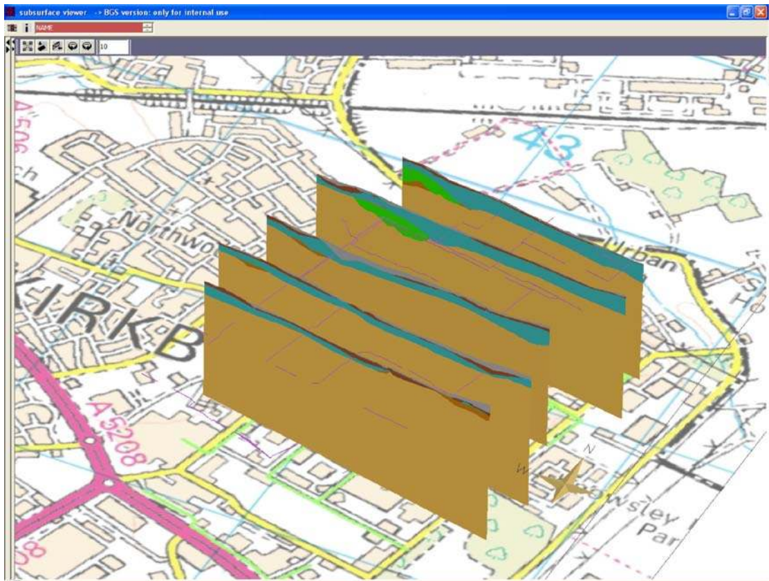
Figure 15. Synthetic cross-sections derived from the Knowsley 3D geological model intersected by buried sewerage network (pink lines). Sherwood Sandstone (orange), Till (blue) Sand (brown) and sand and gravel (green). Model presented in the Subsurface Viewer. OS topography © Crown Copyright. All rights reserved. 100017897/2009
