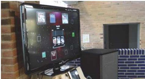
Figure 14. Shared 42” display in the MEET ecosystem. The song in the middle is currently playing. Nominated songs float around the edges and grow in size as they are voted for
