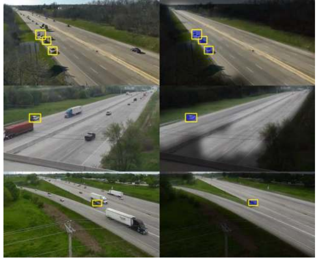
Figure 4. The traffic anomaly dataset containing traffic anomalies caused by vehicle crashes and stalled vehicles. The left column shows detected anomalies in the original frames. The right column presents background modeling results [25].
