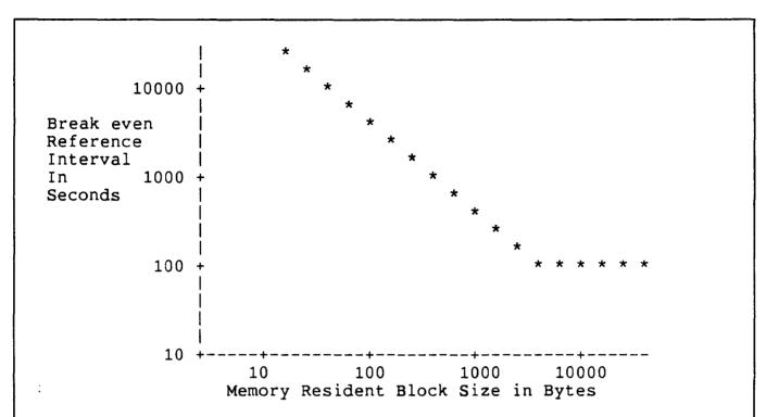
A log-log graph of the break even reference interval (RI) vs the size (B) of the block being stored in main memory. This is computed for 1986 Tandem disc and memory prices. Notice that beyond Bmax (the maximum disc transfer size) the block size does not affect the reference interval.
