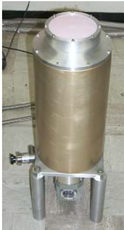
Fig. 6. Vacuum window installed on the LNA assembly.
