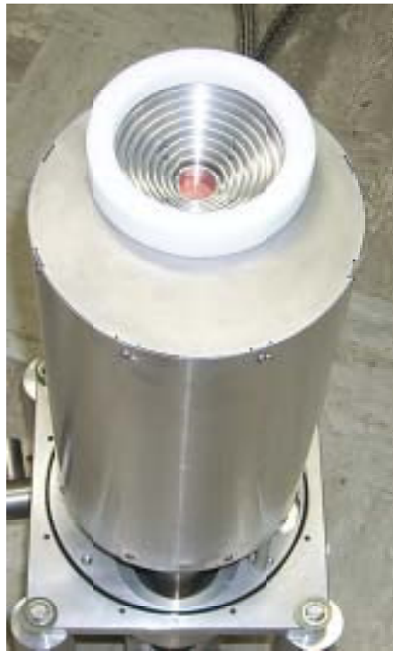
Fig. 5. Radiation shield installed.
