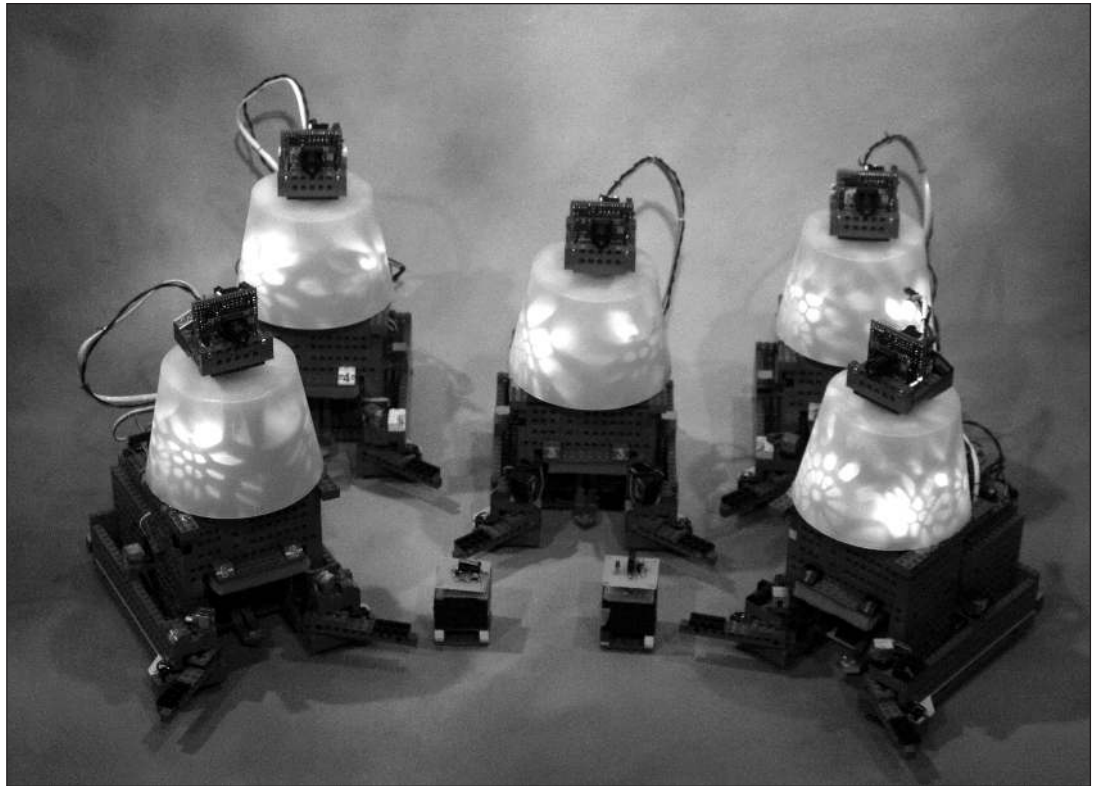
Figure 8. Minnesota's MINDART Is a Test Bed for Evaluating Distributed Robot Control Strategies.
