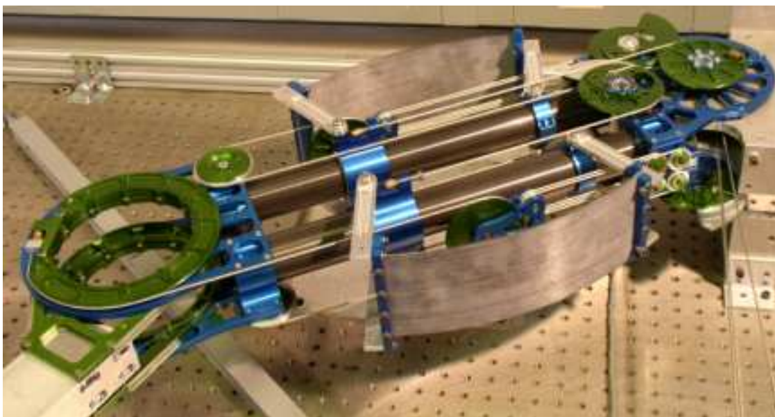
Figure 1: An Actuator with Mechanically Adjustable Series Compliance (AMASC)
