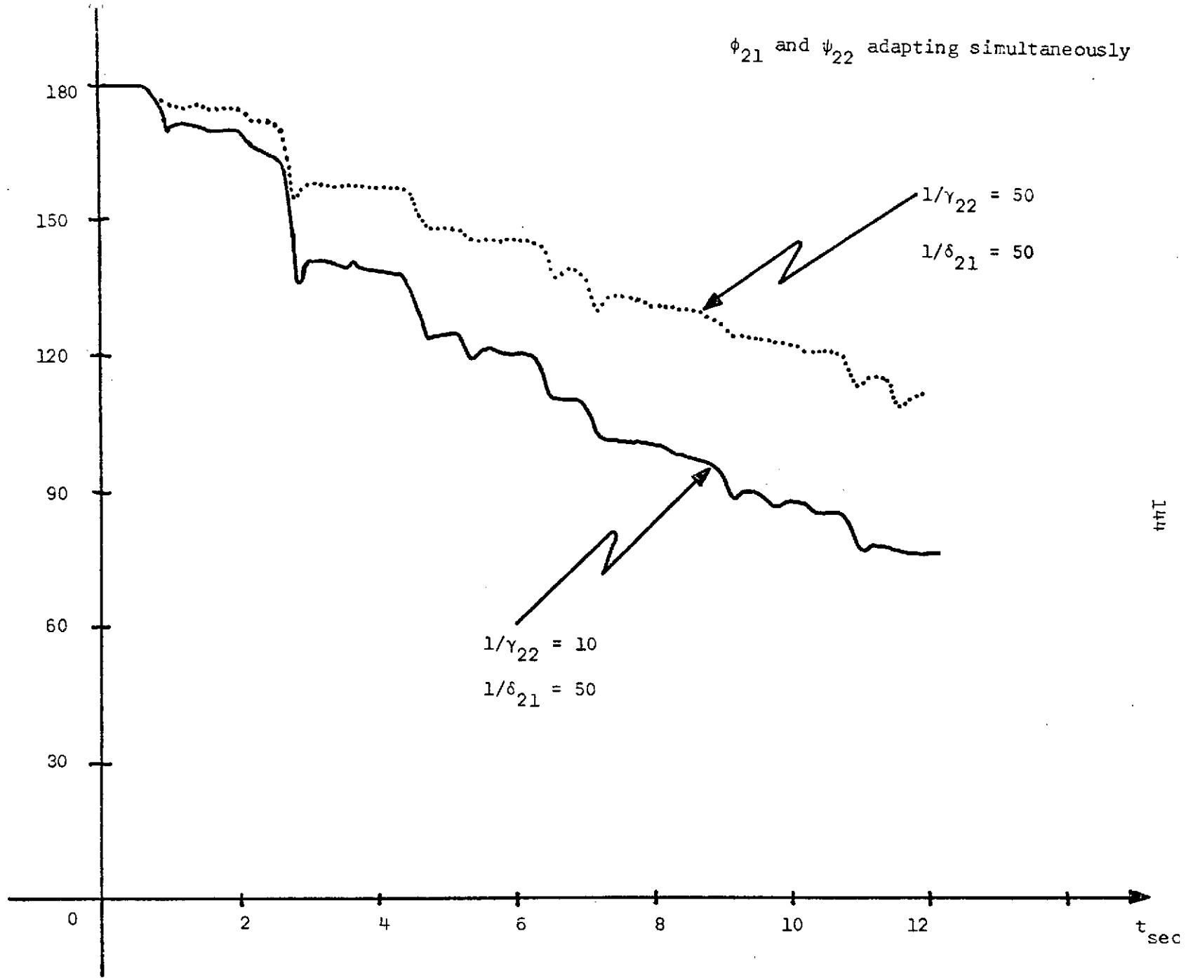
Figure 7.5 Dependence of Rate of Response of \phi_{21} upon Gain Ratios
