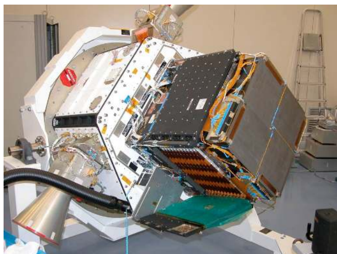
Fig. 9. The AGILE “Payload Unit” consisting of the integrated instrument (here shown without the anticoincidence system during integration tests) and the upper part of the satellite (November 2006).
