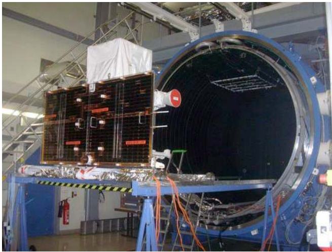
Fig. 13. The AGILE satellite being moved into the thermal-vacuum test chamber in IABG (Munich) (July 2006).
