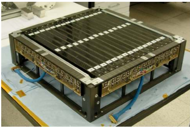
Fig. 7. The MCAL detector consisting of two planes of CsI bars enclosed in carbon fiber supporting structure is shown during the integration process with the signal readout diodes and FFE in the Thales-Alenia Space laboratories in Milan (February, 2005).
