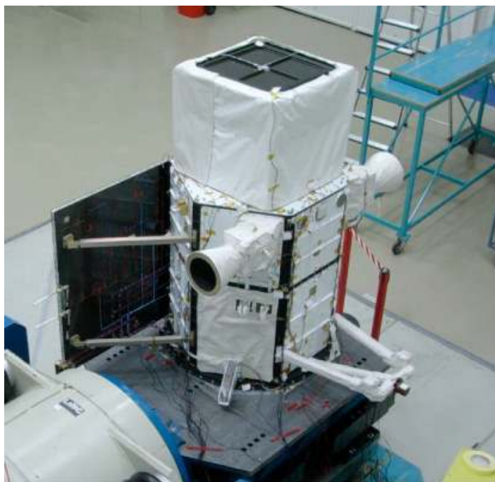
Fig. 2. The integrated AGILE satellite in its final configuration being covered by the thermal blanket during the qualification tests in IABG (Munich), July 2006. The total satellite mass is equal to 350 kg.
