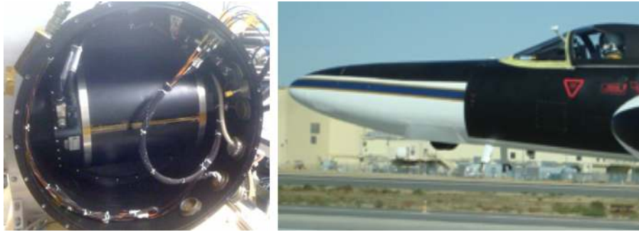
Fig. 1. Left panel: pressure vessel and cylindrical drum housing the AirMSPI camera. Right panel: AirMSPI installed in the nose of the ER-2. The instrument is visible protruding below the fuselage.
