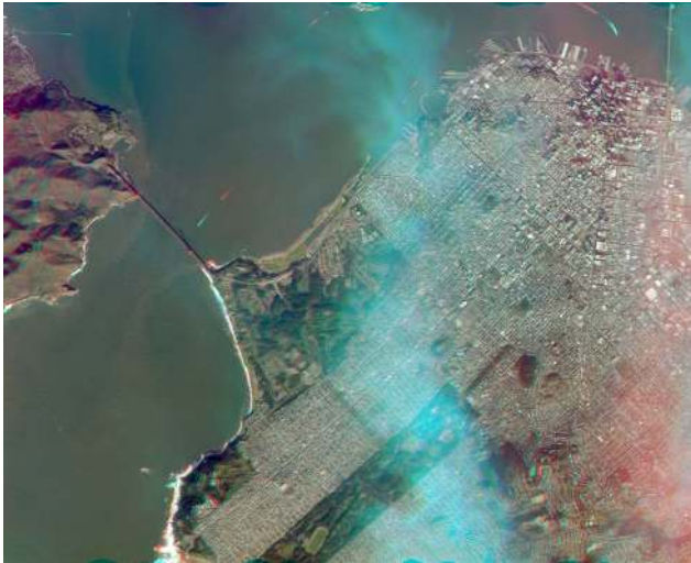
Fig. 16. Stereo anaglyph of San Francisco and a high-altitude cloud field generated using AirMSPI imagery at two view angles (approximately 4^\circ forward and 28^\circ aftward of nadir), acquired on 6 January 2012. 660 nm data from the near-nadir view are displayed in red; 445 and 555 nm data from the aftward view are displayed in blue and green. The image is best viewed using red/cyan glasses with the red filter over the left eye to obtain a 3-D effect. The cloud parallax is too large for good image fusion, but surface topographic relief is apparent when the image is viewed with stereo glasses. North is toward the upper left. The motion of a boat approaching the Golden Gate Bridge is apparent due to the time lapse between the two images used to construct this anaglyph.
