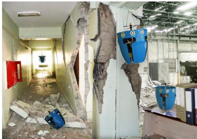
Fig. 1. The AirBurr robot (depicted in the above artist's impression) will be able to explore cluttered indoor environments autonomously. A contact-sensitive structure allows the robot to navigate around obstacles by flying away from them once it touches them. During collisions, the structure protects the robot from damage. If the robot falls to the ground, it can actively upright itself thanks to its legs and take off again without human intervention.
