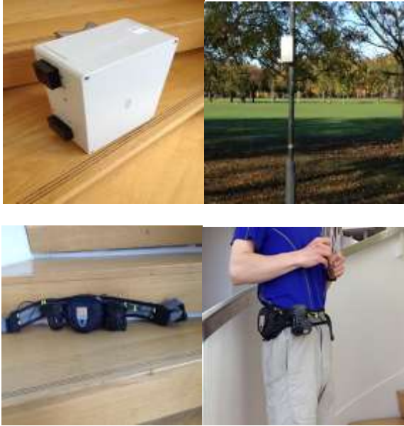
Fig 1. (Top-left) AirSpeck-S monitor attached to a lamp post in the Meadows area in Edinburgh (Top-right); (Bottom-left) AirSpeck-P monitor worn as a belt (Bottom-right).
