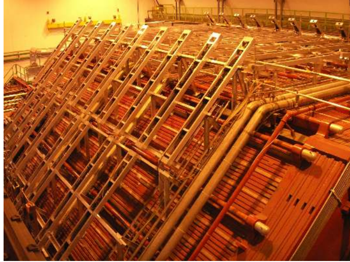
Figure 3.64: Photograph of the ACORDE scintillator module array on the upper faces of the magnet yoke in the ALICE pit. An ACORDE module unit includes two overlapping scintillator counters, each with 190 \times 20 \text{ cm}^2 effective area, and 10 mm thickness, plus two PMTs placed at the end of each scintillator, with optic guide and iron magnetic shielding. All components are attached to an aluminium structure, assembling a 40 kg robust box. There are twenty modules on each one of the three upper faces.
