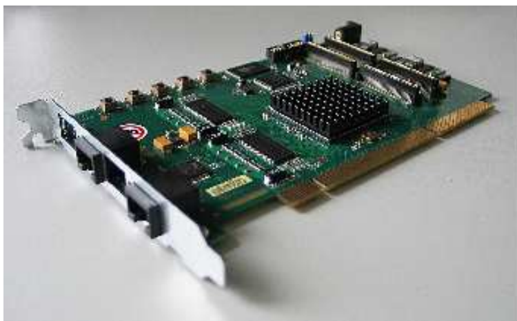
Figure 6.8: H-RORC data pump and FPGA coprocessor.
