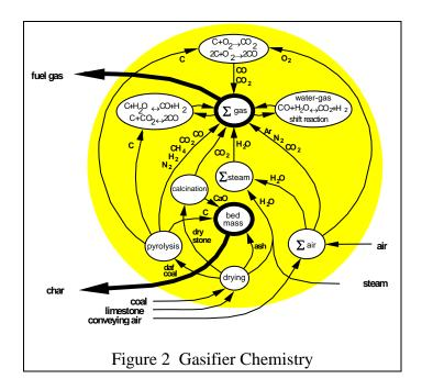
At the global level, there is an overall heat balance for gases and solids to obtain the specific enthalpy of the gas and the total enthalpy of the solids. This model has been validated using measured time histories from the British Coal experimental test facility and it was shown that the model predicts the main trends in fuel gas quality, i.e. calorific value or CV in Figure 3.
