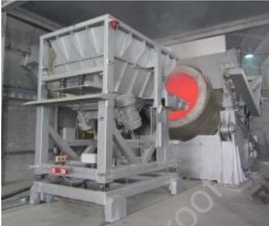
Figure 33: A vibratory charging machine, reproduced from [182].
