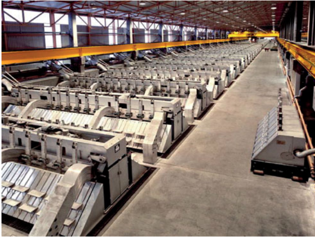
FIGURE 1. A modern potline with high-amperage side-by-side prebake cells.
