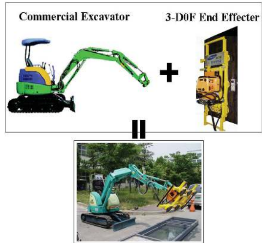
Fig. 9. Concept of curtain-wall installation robot
