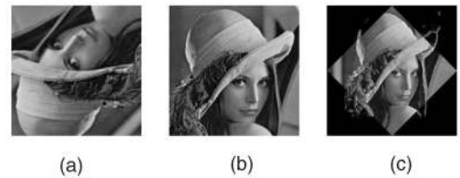
Fig. 10. Registration of images with noncorresponding parts. Image (a) is aligned to image (b). (c) is created by aligning (a) to (b). The edges in (b) are detected and overlaid on the aligned image (a).
