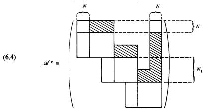
Again, a' can be inverted efficiently by Gaussian elimination with partial pivoting. The amount of fill-in introduced is indicated by the shaded areas in (6.4). The leading term in the operational count is  $I\{N_1[N_1^2/3 + 3N_1N/2 + 2N^2]\}$ .
