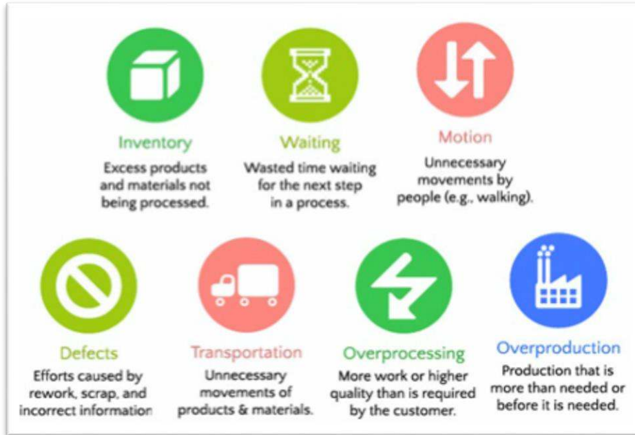
Figure 2.1. The Seven Deadly Wastes. Reprinted from The Definitive Guide to Waste Reduction for Manufacturers, on MFC.com by A. Carpenter, submitted by B. Defoor, March 16, 2015, Retrieved August 9, 2016 from http://www.mfg.com/blog/definitive-guide-waste-reduction-manufacturers . Copyright 2016 by MFG.com.
